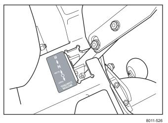
Steering controls in the outward, locked neutral position
